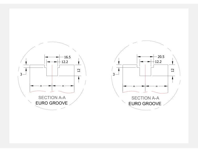
Typical faceplate widths are 16mm or 20mm, this is measured across the face of the lock.
